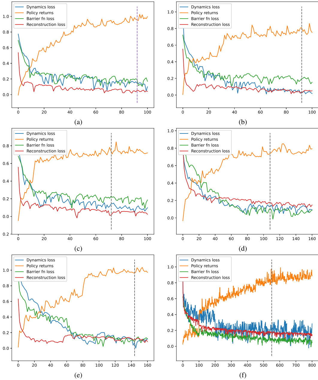
Figure 6: Training plot for the given 6 tasks with losses or returns from individual elements. x-axis is number of episodes and y-axis is the magnitude of individual metrics. (a) Car trajectory tracking Kinematic model (b) Car trajectory tracking Sideslip model (c) 3D Quadrotor (only sensor data) (d) 2D Quadrotor with obstacles (e) 3D Quadrotor with an obstacle (f) LatentCBF based Interfuser with CBF on Carla leaderboard
