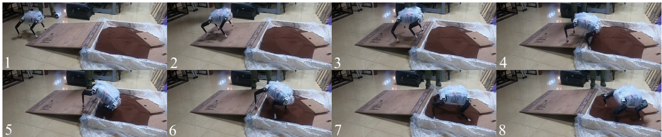
Fig. 5: Shown at the top are the plots of variation in Torso Orientation, Slope Orientation, and Tracking Errors of foot trajectory. And at the bottom keyframes of the hardware experiment performed on slope of 9^\circ and loose terrain made of artificial sand are shown
